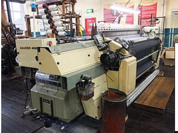
Production Loom Sauer 400S Rapier Loom (1980)
