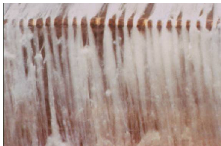
Carding a fiber web. Lengthwise direction orientation of fibers.
