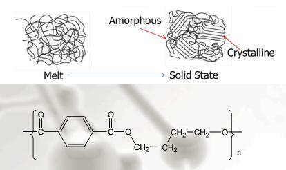
The PBT polymer can be processed to have high crystallinity – typically as high as 60% – giving it many useful properties such as high hardness, stiffness, strength and chemical resistance.
