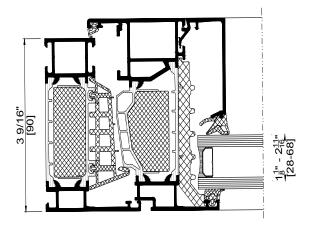
Horizontal section detail of Schüco Window System AWS 90.SI+ fixed window
