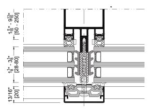
Horizontal Section of Schüco Facade System FWS 50.SI Green with PVC-U pressure plate
