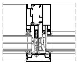
Horizontal section detail of the Schüco Facade System FWS 60 CV.HI
