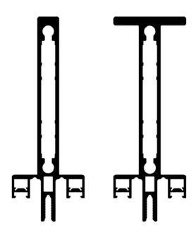
Horizontal section detail of Schüco Facade System FWS 50 S
