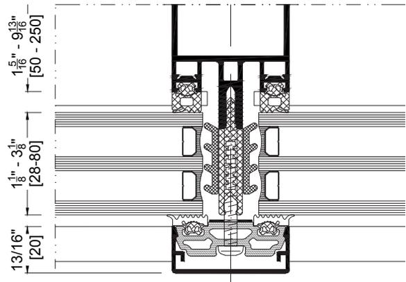
Horizontal Section of Schüco Facade System FWS 50.SI Green with PVC-U pressure plate
