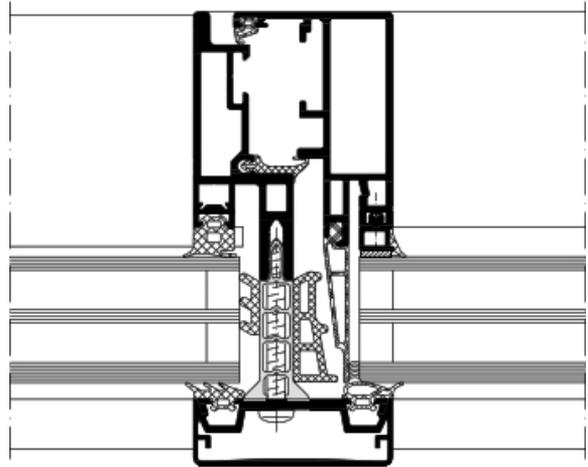
Horizontal section detail of the Schüco Facade System FWS 60 CV.HI
