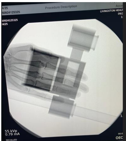
Figure II.1: Xray Image Depicting Center Chest Support Block Radiolucency
