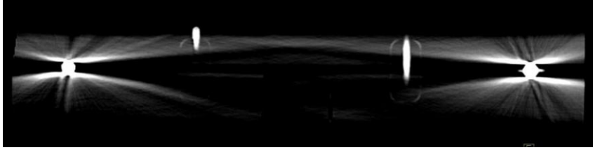
Figure 11.9: Another Cat Scan Image that Shows Only Metal Components Cause Scattering
