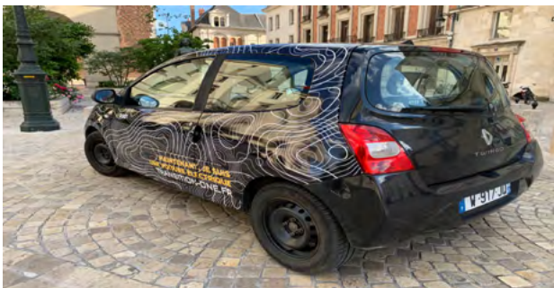
Figure 6: Transition-One electric Renault Twingo II conversion 120
