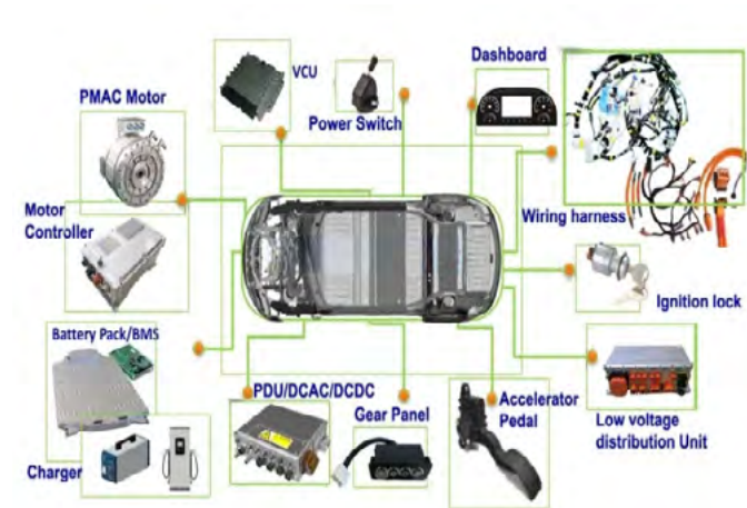
Figure 5: Basic components for LDV electric retrofitting, Zemo, 2021
