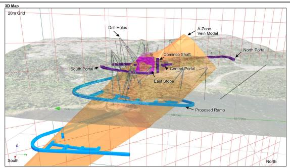
The images to the left are three dimensional representations of the A-Zone with drill hole traces in dark grey and existing workings in purple.
