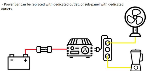
Note: The above scenario might be modified to have a dedicated sub-panel and associated outlets in place of the power bar or extension cord to the inverter.
