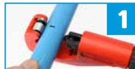
**Cut Pipe to length** with tubing cutter (cut must be square) (DO NOT USE HACK SAW)
