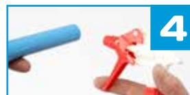
**Wet end of pipe** with very diluted soapy water (DO NOT USE ANY OIL OR GREASE LUBRICANT)
