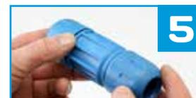
**Loosen FITTING CONE NUT PARTIALLY** (LOOK INSIDE EACH FITTING FOR INNER PARTS (inner parts, o-ring, stainless steel bite ring))
