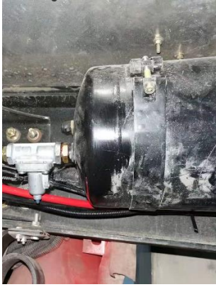
1 . 2 Pressure protection valve to control box air intake, 6x4 air tubing.
