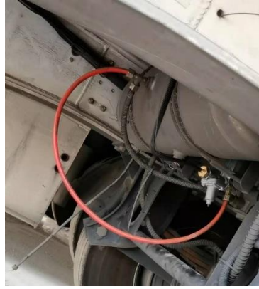
1 . 2 Pressure protection valve to control box air intake, 6x4 air tubing.
