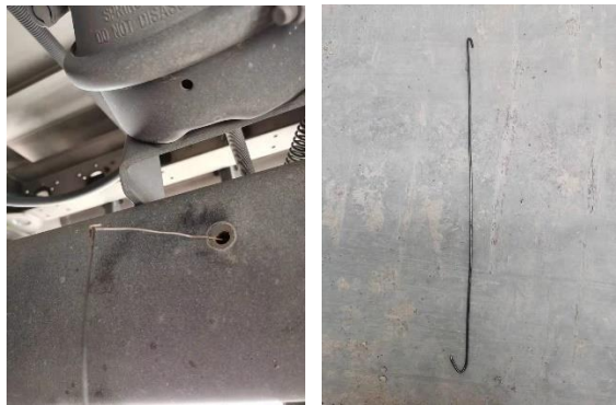
Figure 23: The air tubing inside the axle tube, with a spring protective sleeve.
