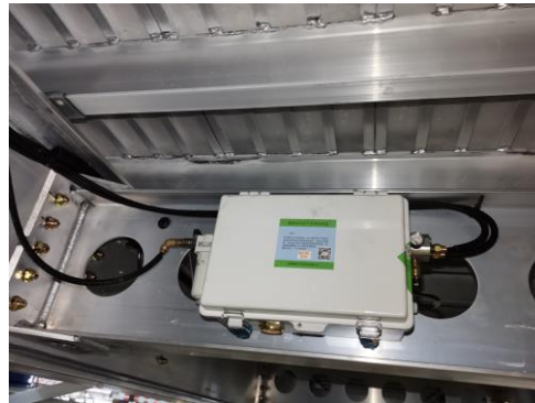
Figure3 9/40: Where the control box is installed. Normally at the rear of the beam, find the right position to drill 4 holes of diameter 10.5mm, equipped with 4 sets of flat washers, cushions, nuts, tighten to 22-30Nm. At least 5CM clearance under the vents to facilitate the air exhaust.
