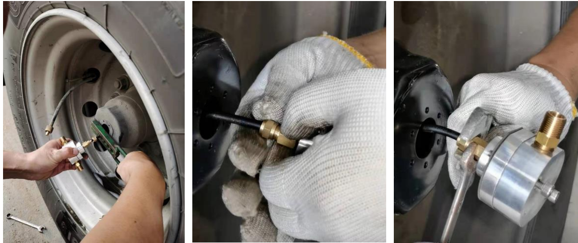
Figure 27/28/29: Connection of rotary union to air tubing / installation of quick screw nut / tightening of quick screw nut
