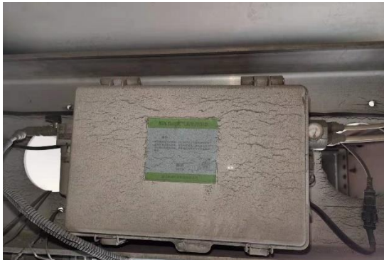
Figure3 9/40: Where the control box is installed. Normally at the rear of the beam, find the right position to drill 4 holes of diameter 10.5mm, equipped with 4 sets of flat washers, cushions, nuts, tighten to 22-30Nm. At least 5CM clearance under the vents to facilitate the air exhaust.
