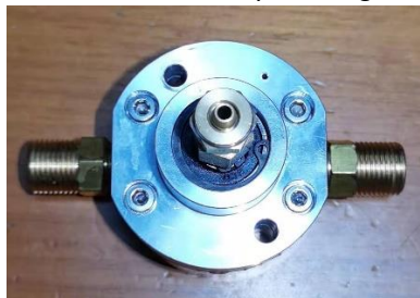
Figure4/5/6: Single-tire rotary union /Dual tire rotary union/ gasket for V2.0
