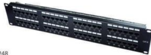
S/N : LE-P3248 Description: 19" 2U 48Port CAT5E/CAT6 UTP with cable Management Packing data: 20EA/ctn Packing size (mm): 53x26.3x51
