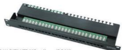
S/N : LE-P3209 Description: 19" 1U CAT3 UTP 8P4C 50Port Krone IDC 90° Packing data: 20EA/ctn Packing size (mm): 53x26.3x51
