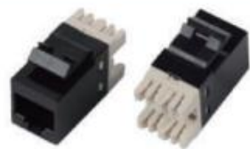
S/N : LE-K2027-C6 Description: CAT6 UTP Dual IDC 180° Packing data: 1000EA/ctn Packing size (mm): 42x26.3x45
