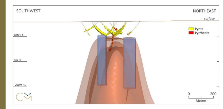
Bradbury's Prospect Long Section looking North-West Drillholes – Trace width = highlighting increasing magnetic susceptibility at depth. Buff coloured shapre = Original 3D magnetic inversion model, darker (blue) colout = Subsequent forward model profiles.
