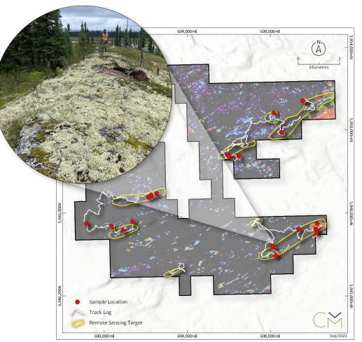
Carmoy Property – Remote Sensing Target Areas and identified pegmatite dyke (inset). Map is annotated with Coolabah field team traverses and sample collected within the Carmoy property
