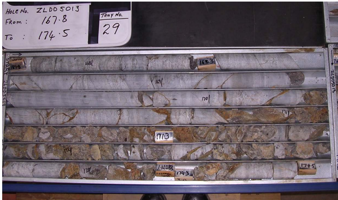
Figure 2 ZLD5013 Broken/faulted zone from 170.8 to 174.5m
