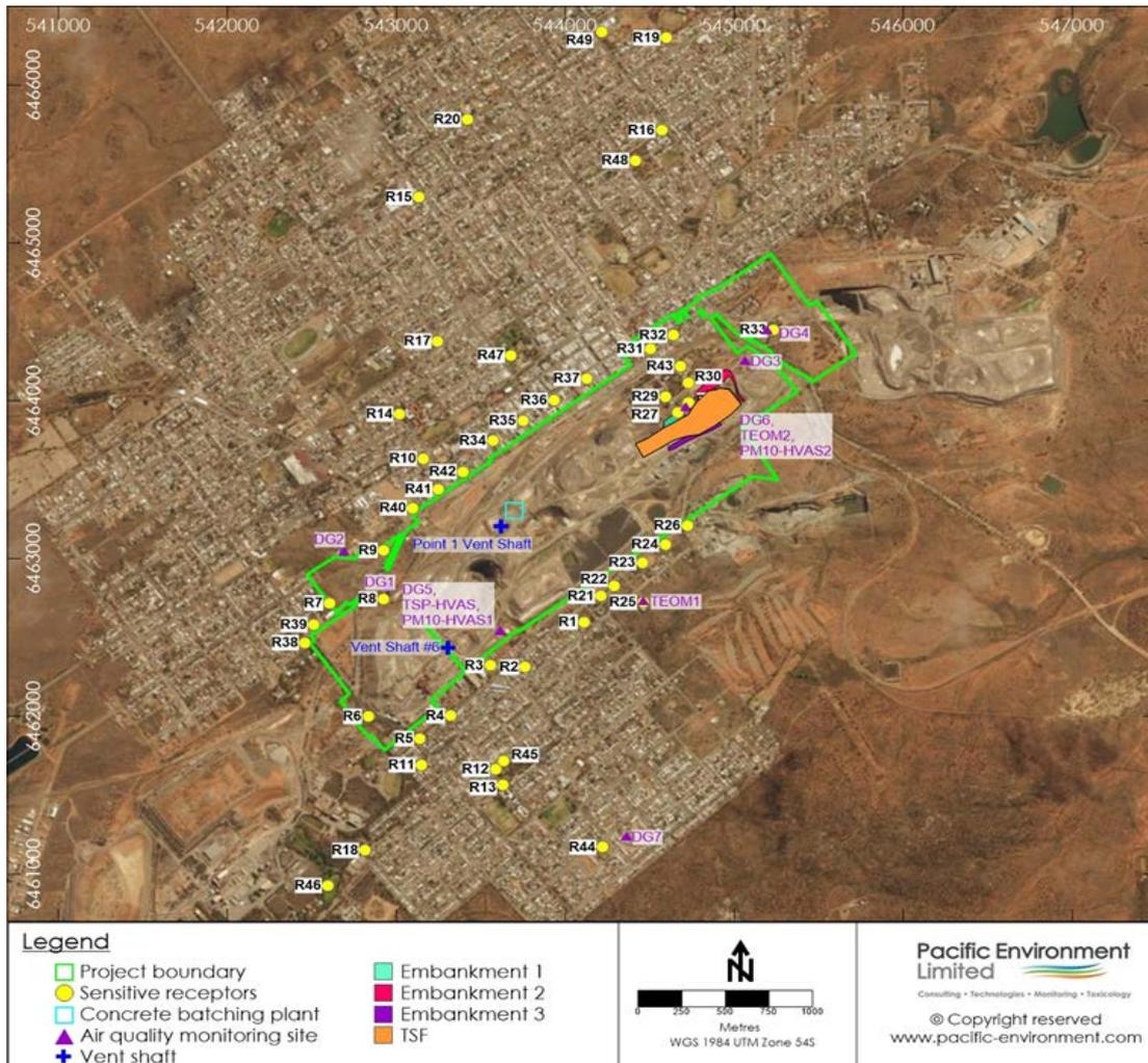
**Figure 2.1: Location of proposed Concrete Batching Plant, Tailings Storage Facility Embankments 1-3 and air quality modelling locations (i.e. sensitive receptors).**
