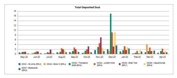
The dust levels recorded in Dust Gauges in April 2023 were lower than previous months. The highest dust levels were recorded in the D4 Junction Mine gauge. The predominant wind direction for April was from the South as shown in the Wind Rose in Section 4. This result is likely caused by dust from the rail yard.
