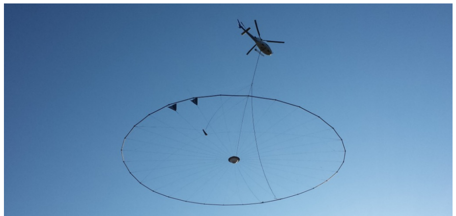
HelITEM 2 helicopter time-domain AEM Survey
