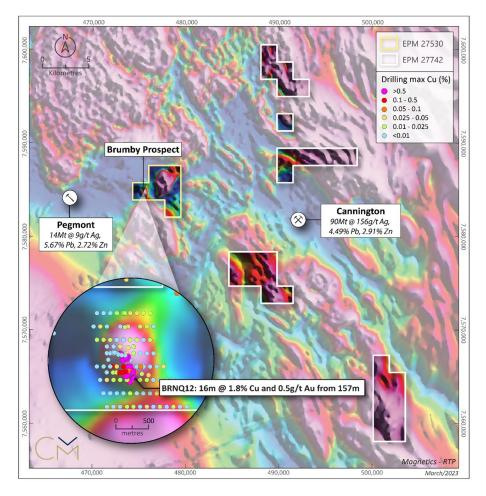
**Figure 5:** Cannington Project – Overlayed on Regional Magnetics (RTP). Inset shows drillhole collars coloured by maximum downhole copper values.
