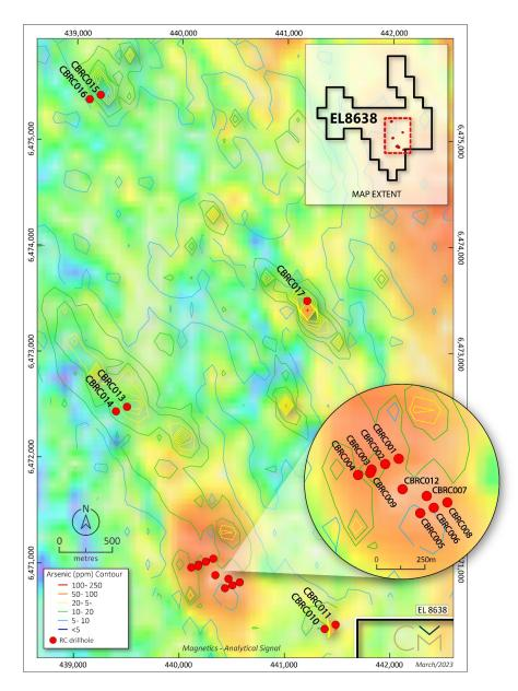
Figure 2: Bradbury's Prospect - Completed RC holes over government AIG magnetics and contoured soil arsenic (ppm).
