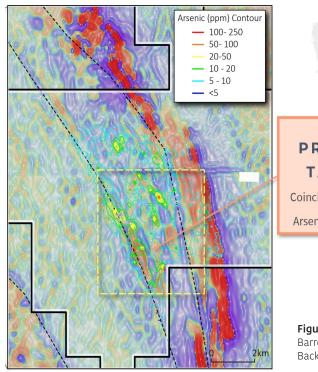
PRIORITY TARGET Coincident Magnetic + Arsenic Soil Anomaly
