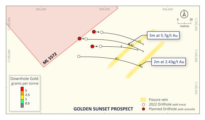
Figure 2: Golden Sunset Prospect plan view with downhole Au g/t projected to surface
