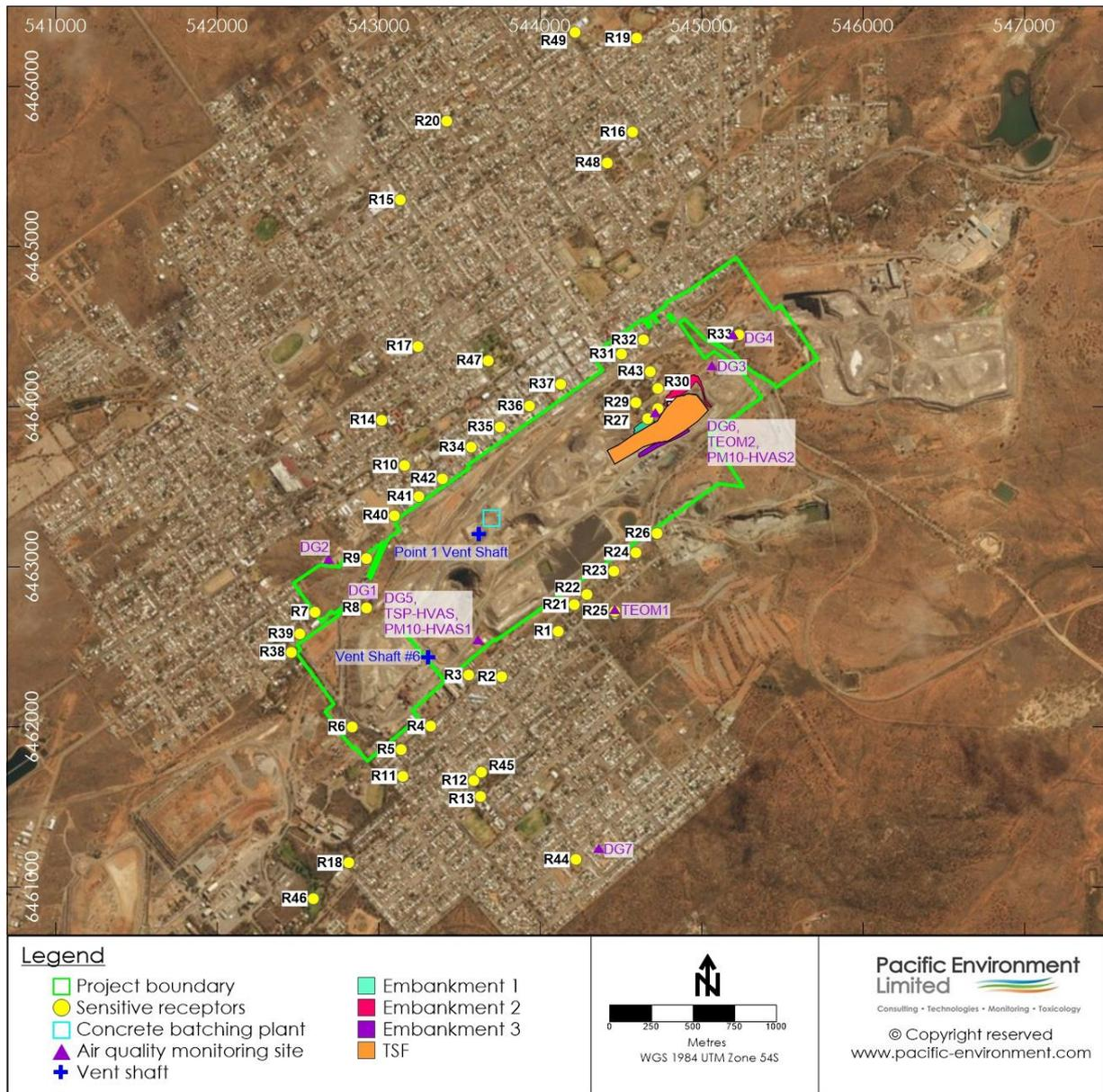
Figure 1-1: Location of proposed Concrete Batch Plant, Embankments 1, 2 and 3, sensitive receptors and air quality monitoring network
