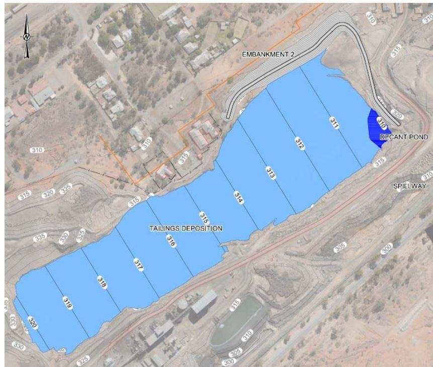
Figure 2: Stage 1 Intermediate Tailing Deposition
