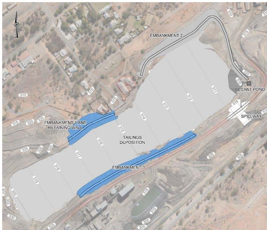
Figure 3: Stage 2 Embankment 1 and Embankment 3 Construction
