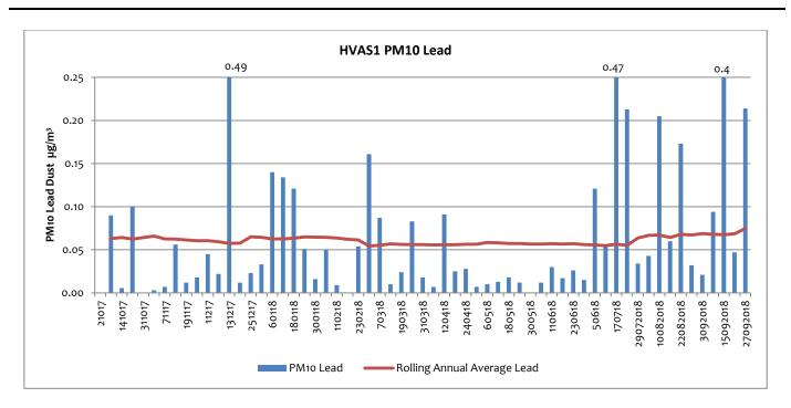
Lead levels were elevated on 15 and 27 September which was consistent with the high winds on these days. Dust suppressant is applied to free areas on site and roads are continually watered using water carts.
