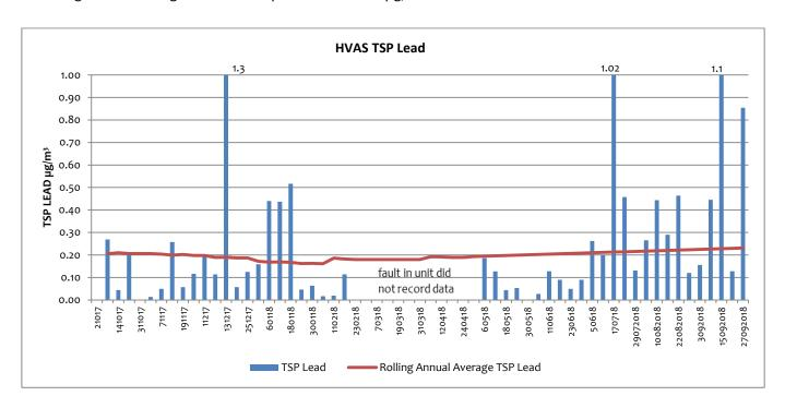
Lead levels were elevated on 15 and 27 September which was consistent with the high winds on these days. Dust suppressant is applied to free areas on site and roads are continually watered using water carts. The rolling annual average for TSP Lead to September is  $0.23 \, \mu g/m3$ .
