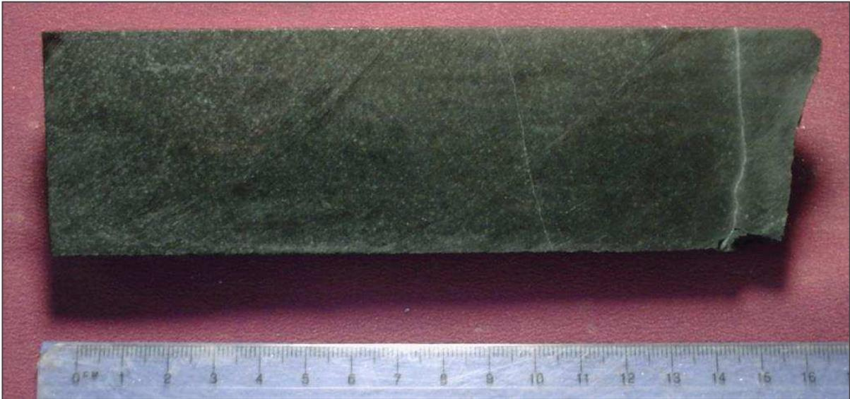
Figure 4-4: Image of Dolerite Sample
