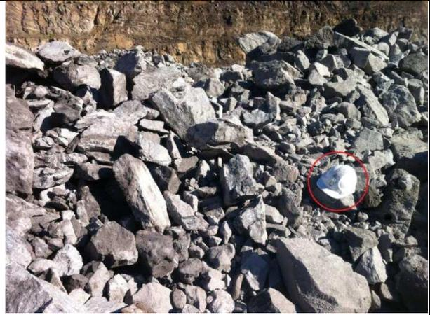
Photo 2: Another area of the waste rock stockpile with hard hat for rock size reference
