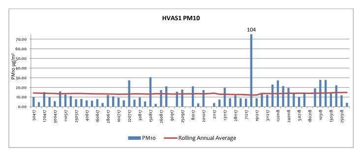
The HVAS1 monitoring unit is located on the Rasp Mine and the limit criteria do not apply at this point, criteria apply at the closest residential location. The recorded annual average for  $PM_{10}$  to March is 14.5  $\mu g/m^3$  which is below the  $PM_{10}$  annual average criterion of 25  $\mu g/m^3$  required at the nearest residential location. Overall the trend for  $PM_{10}$  at this location remains consistent with the previous 12 months.
