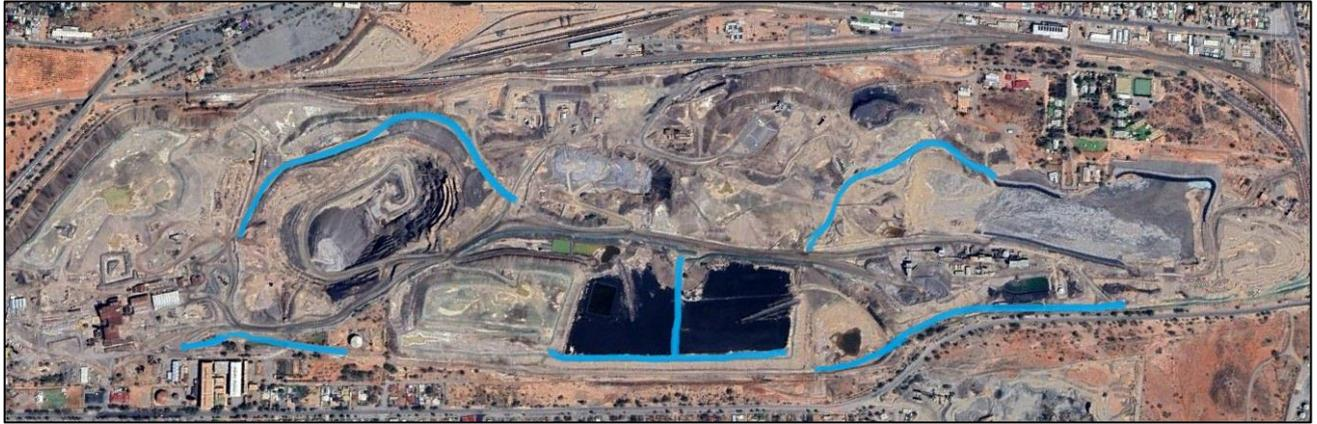
**Figure 4-3 Unsealed roads treated with dust suppressant**
