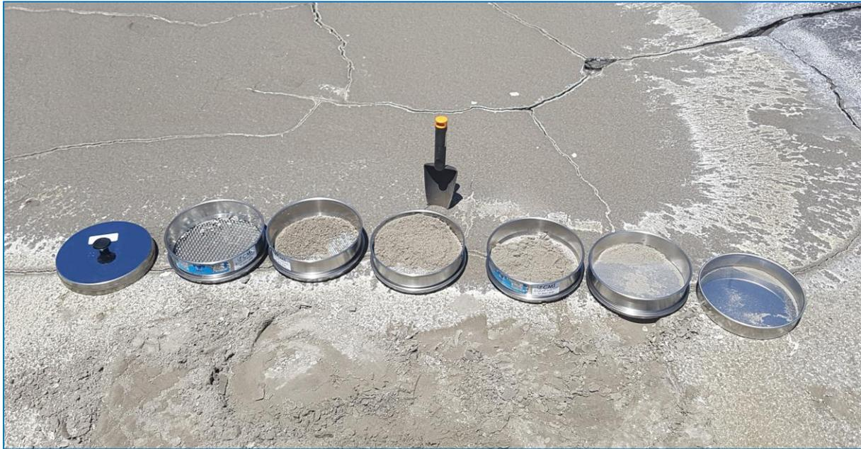
**Figure 3 - Example of the USEPA sieving method (mode sieve indicated by position of hand trowel)**
