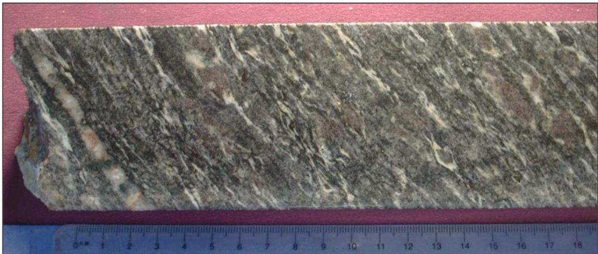
Figure 4-1: Image of Garnet Pelite (GPE) Sample
