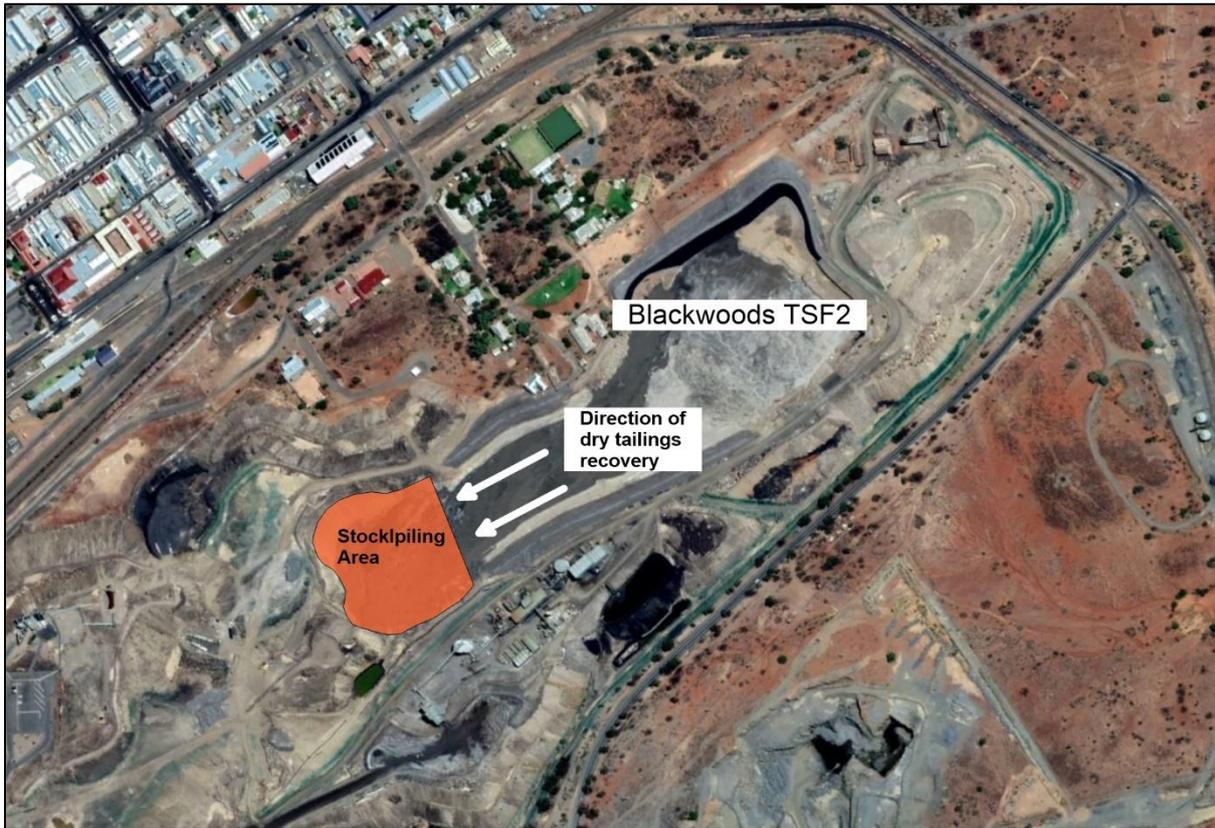
**Figure 2-1: Indicative locations of stockpiling and dry stacking**
