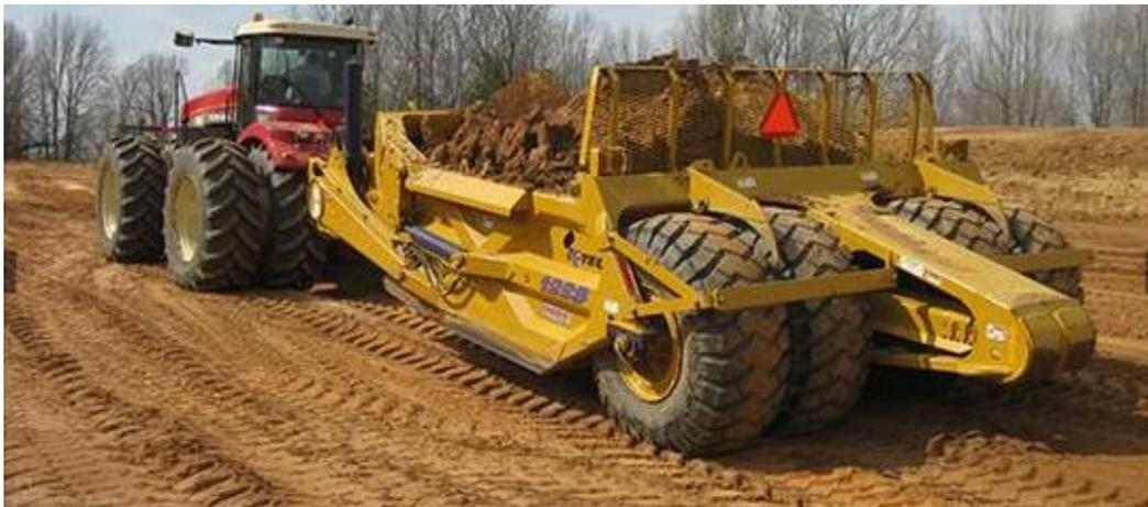
**Figure 5-1: Example of rubber tired tractor scoops proposed for tails harvesting**
