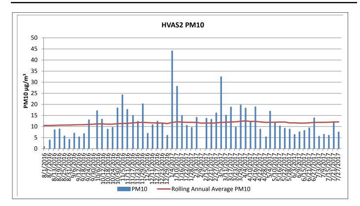
This monitoring unit is located on the Rasp Mine and no criterion applies at this point, criteria apply to the closest residential location. The annual average  $PM_{10}$  for July of 12  $\mu$ g/m<sup>3</sup> is well below the  $PM_{10}$  annual average criterion of 30  $\mu$ g/m<sup>3</sup> required at the nearest residential location. The Rasp Mine is in compliance with this criterion.
