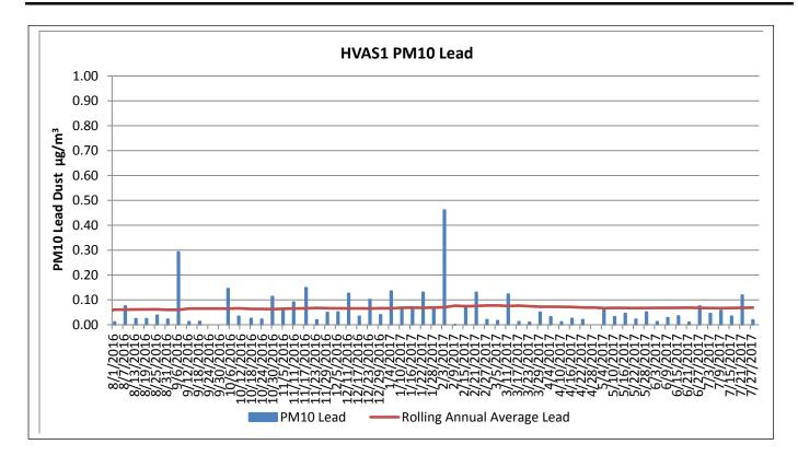
There is no guideline for assessing  $PM_{10}$  lead dust. However, the overall the trend for lead dust at this location remains consistent with the previous 12 months.
