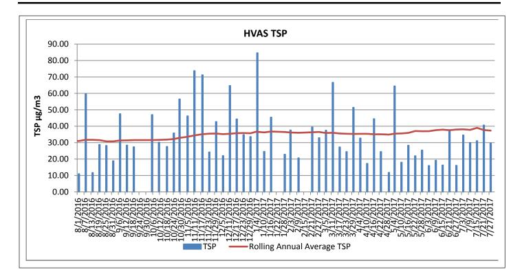
This monitoring unit is located on the Rasp Min and no criterion applies at this point, criteria apply to the closest residential location. The annual average TSP for July of 36  $\mu$ g/m<sup>3</sup> is well below the TSP annual average criterion of 90  $\mu$ g/m<sup>3</sup> required at the nearest residential location.
