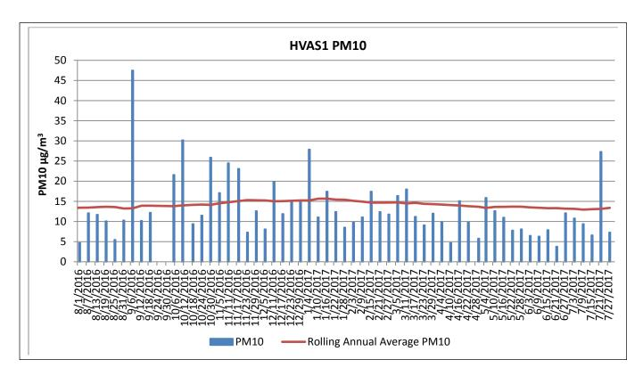
This monitoring unit is located on the Rasp Mine and no criterion applies at this point, criteria apply to the closest residential location. The data indicates that the annual average  $PM_{10}$  for July of 13 µg/m<sup>3</sup> is well below the  $PM_{10}$  annual average criterion of 30 µg/m<sup>3</sup>.
