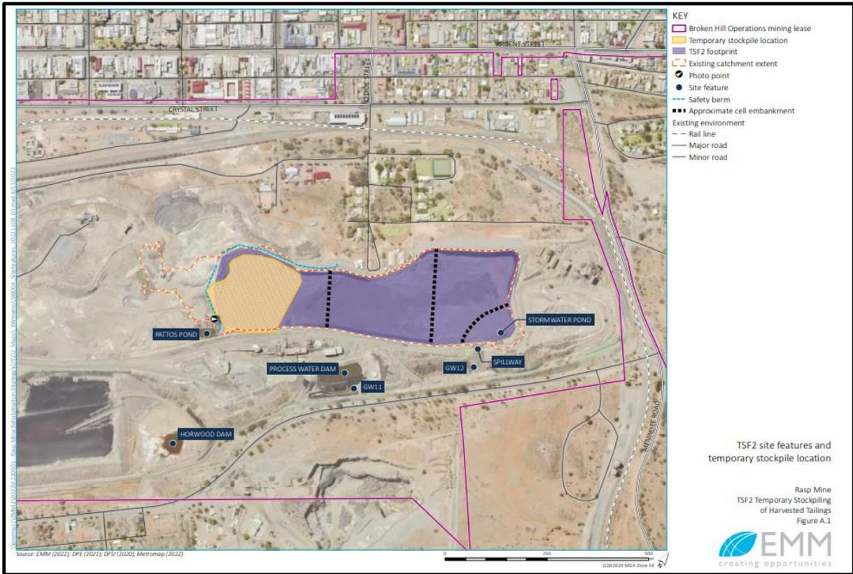
**Figure 4: Temporary Tailings Stockpile**
