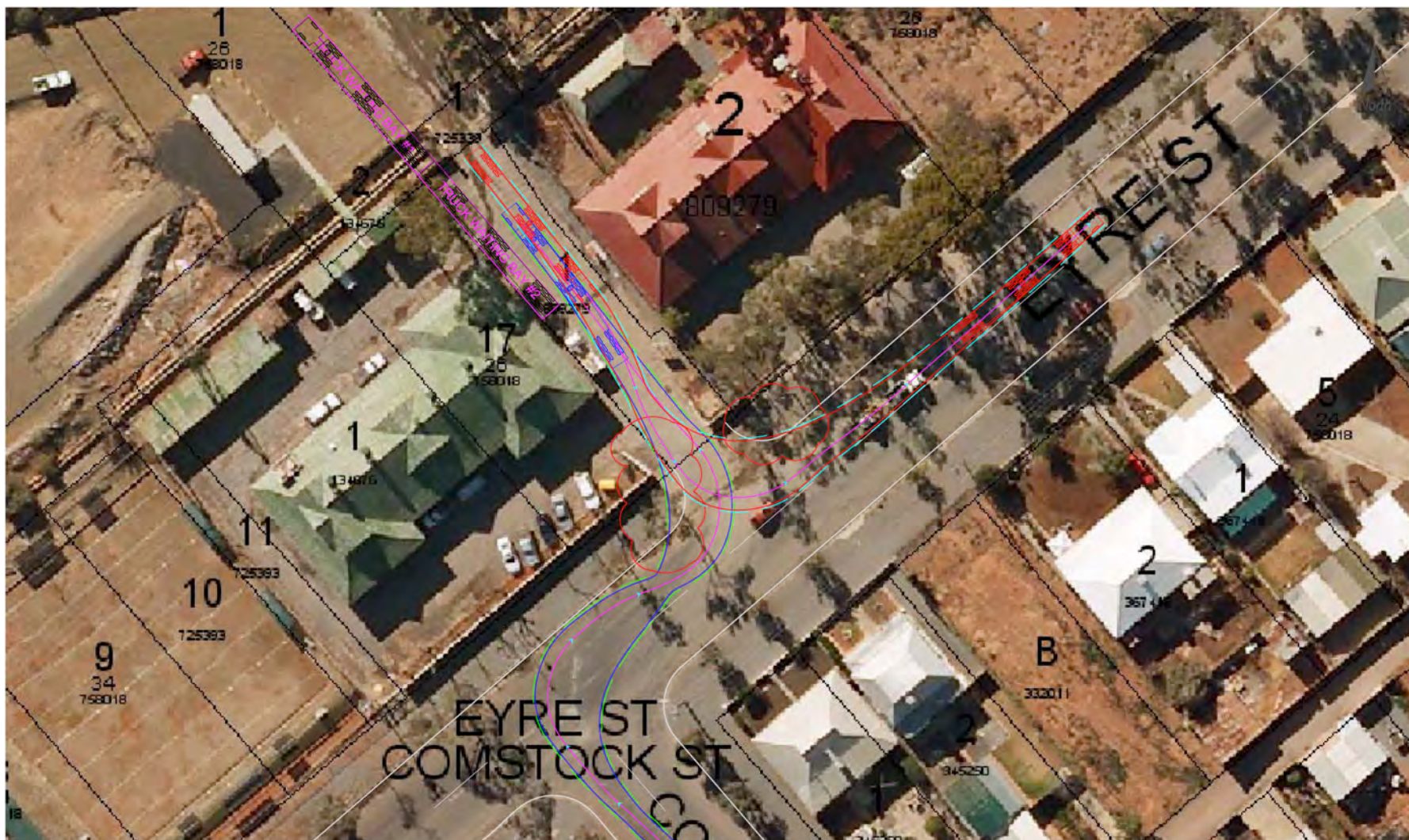
Figure 2-5: Sweep paths for 26m B-double trucks entering / leaving the site
