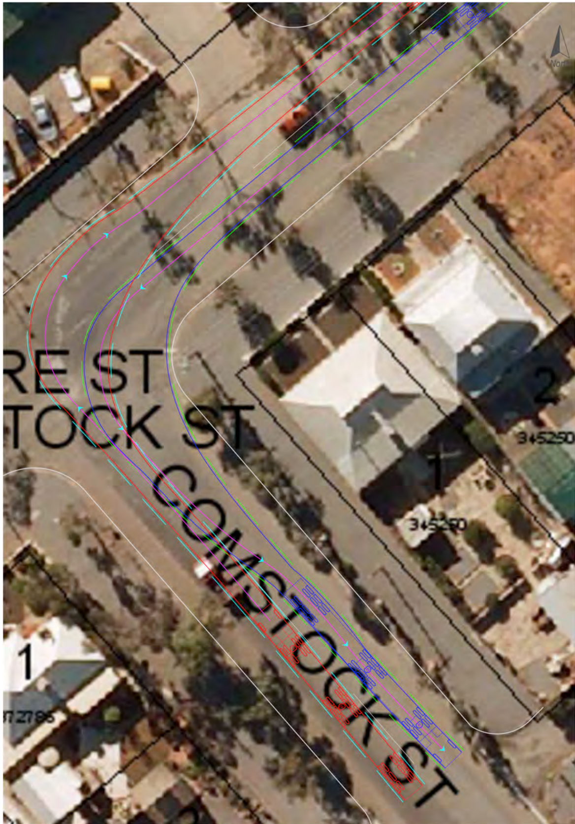
Figure 2-6: Current sweep paths for 26m B-double trucks at the Comstock Street / Eyre Street intersection
