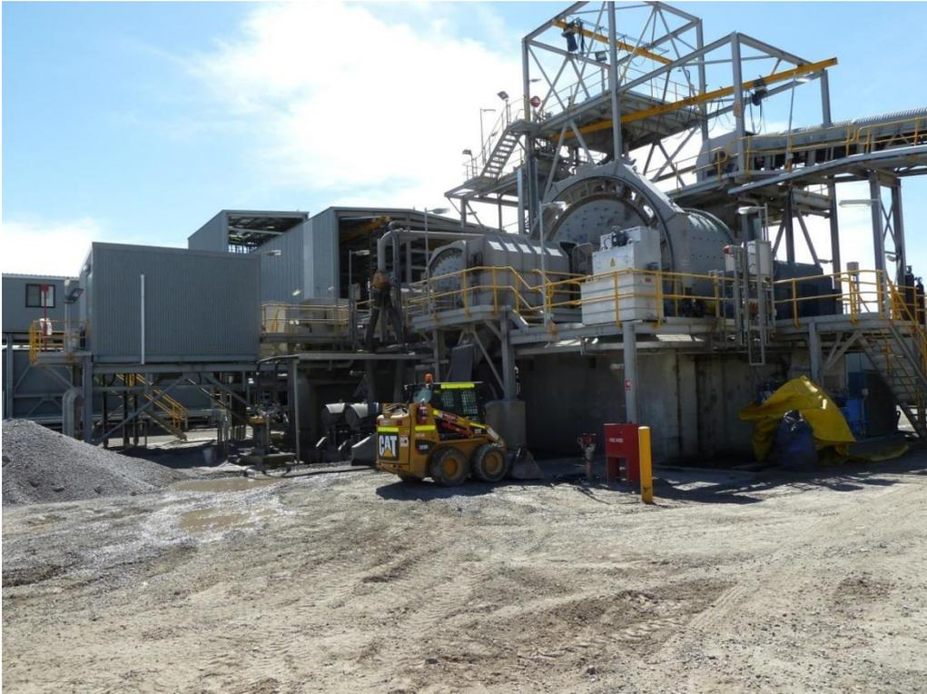
Photo 24. Building installed around the flotation facility providing shielding of the SAG and Ball mills.
