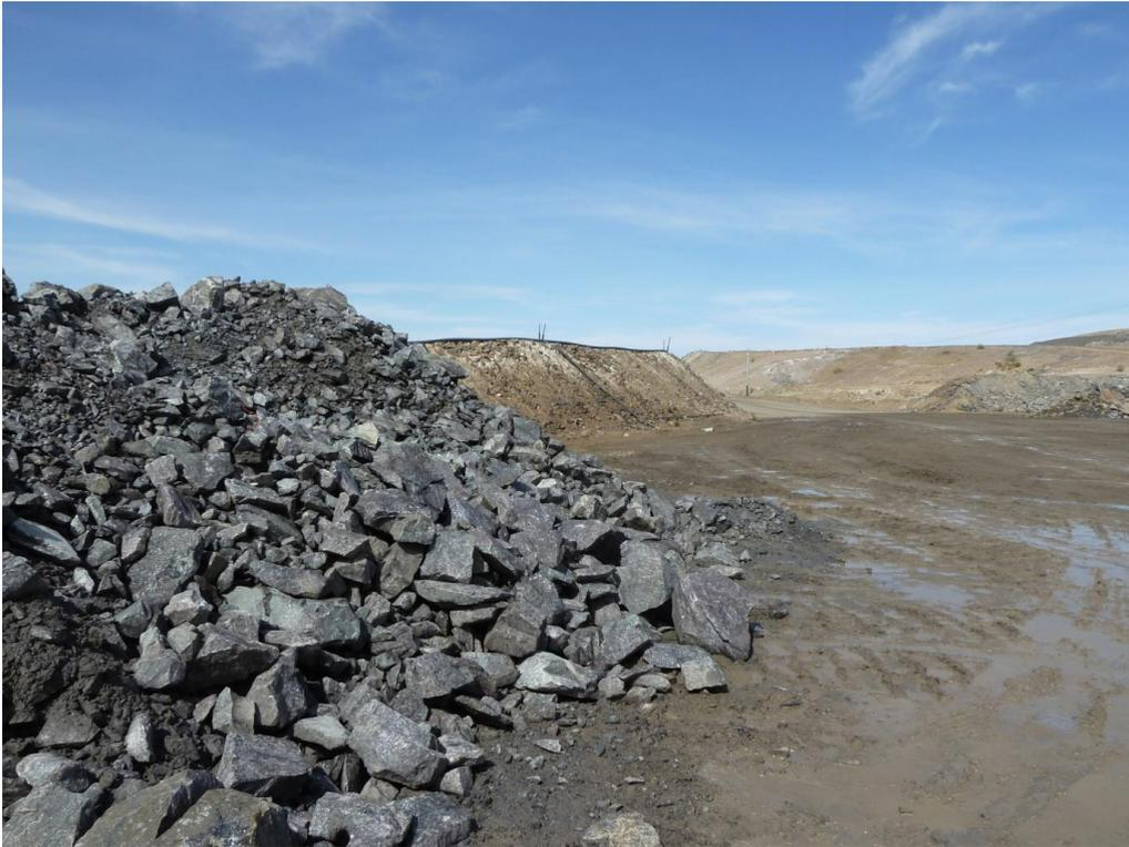
Photo 16. ROM pad showing ore stockpile, bunds and water sprays.
