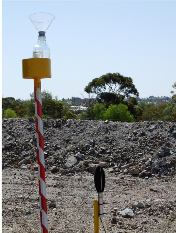
Photo 28. Dust sampling jar on site and microphone for noise monitoring.
