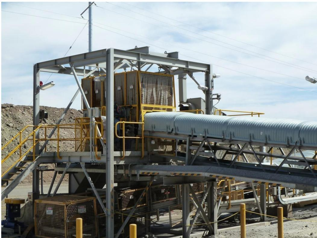
Photo 6. Covered conveyors and enclosed transfer point.
