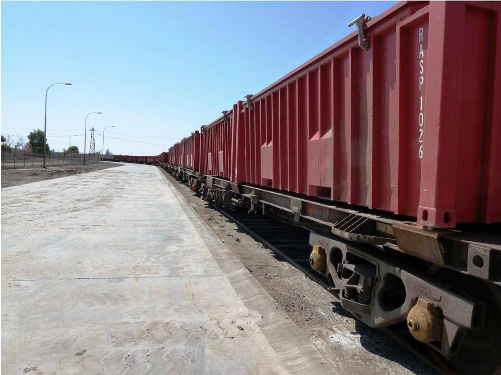
Photo 15. Rail cars loaded with zinc concentrate containers.
