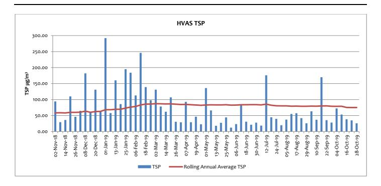
HVAS (EPL10) is located on the southern boundary of Rasp Mine and while limit criteria do not apply at this point, they do apply at the closest residential location. Overall the trend for TSP at this location has risen over the 12 months to October although it has started to trend downwards in the last couple of months.
