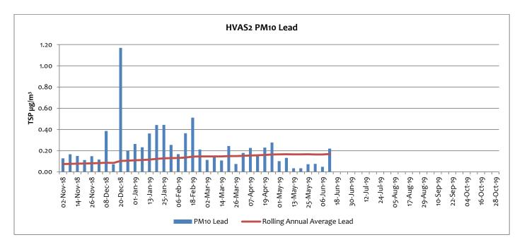
There is no guideline for assessing PM10 lead dust; the Annual Rolling Average for lead dust at this location has increased over the previous 12 months from  $0.07 \,\mu\text{g/m}^3$  to  $0.16 \,\mu\text{g/m}^3$  at the end of June 2019.
