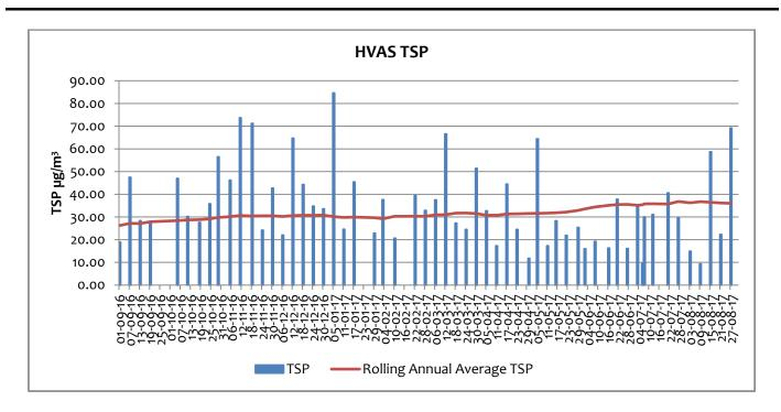
This monitoring unit is located on the mining lease and no criterion applies at this point, criteria apply to the closest residential location. The data indicates that the annual average TSP for August of 35.5  $\mu$ g/m<sup>3</sup> is well below the annual average criterion for TSP of 90  $\mu$ g/m<sup>3</sup>.
