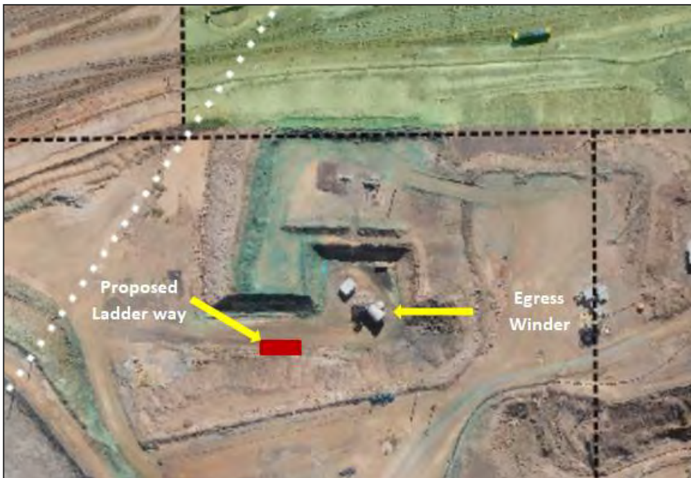
Figure 3.2 Location of emergency egress ladderway in relation to the current egress winder
