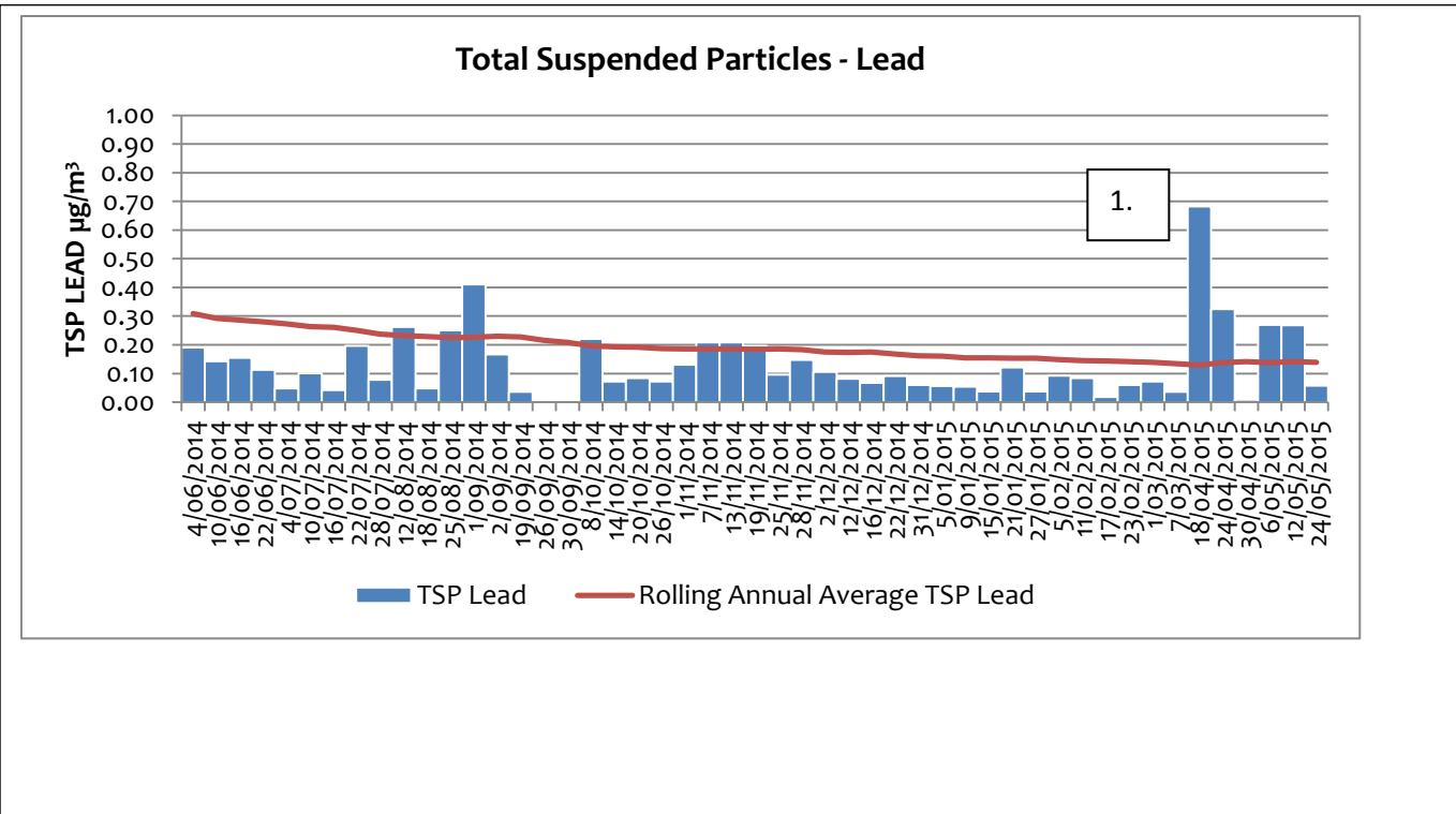
1. Spike on the 18<sup>th</sup> was investigated. Lab QC was okay with no evidence of lab contamination. Wind conditions were not extraordinary and it rained. Field sampling methods have been checked to prevent any sample contamination.
