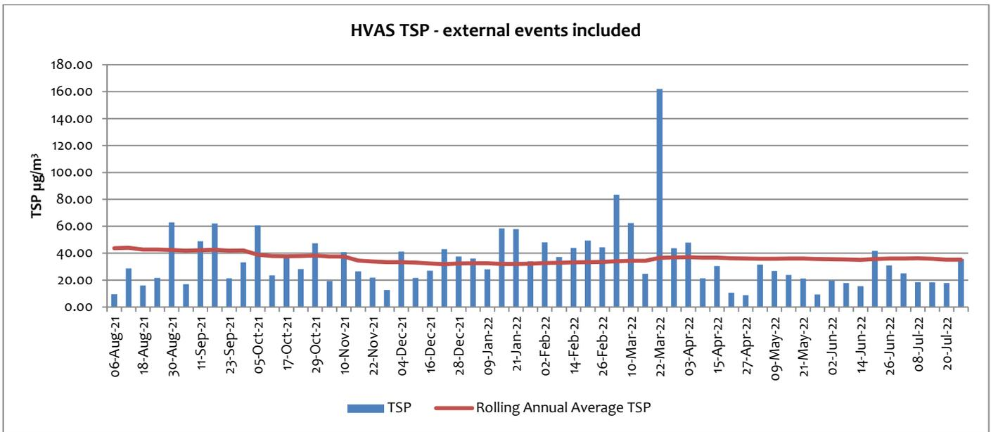
HVAS (EPL10) is located on the southern boundary of Rasp Mine and while limit criteria do not apply at this point, they do apply at the closest residential location.
