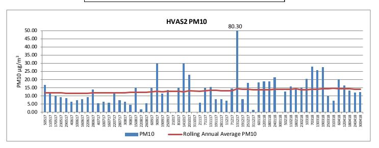
The HVAS2 monitoring unit is located on the Rasp Mine and limit criteria do not apply at this point, criteria apply at the closest residential location. The recorded annual average  $PM_{10}$  to April is 14 µg/m³ which is below the  $PM_{10}$  annual average criterion 25 µg/m³ required at the nearest residential location.
