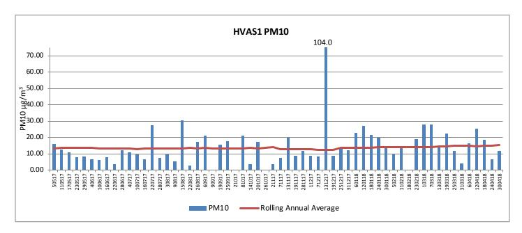
The HVAS1 monitoring unit is located on the Rasp Mine and the limit criteria do not apply at this point, criteria apply at the closest residential location. The recorded annual average for  $PM_{10}$  to April is 15.3  $\mu g/m^3$  which is below the  $PM_{10}$  annual average criterion of 25  $\mu g/m^3$  required at the nearest residential location. Overall the trend for  $PM_{10}$  at this location remains consistent with the previous 12 months.
