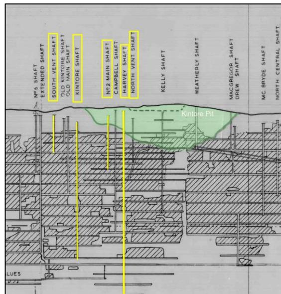
Figure 5- Section View, Intact hangingwall and Footwall surface shaft collar Locations (looking W)
