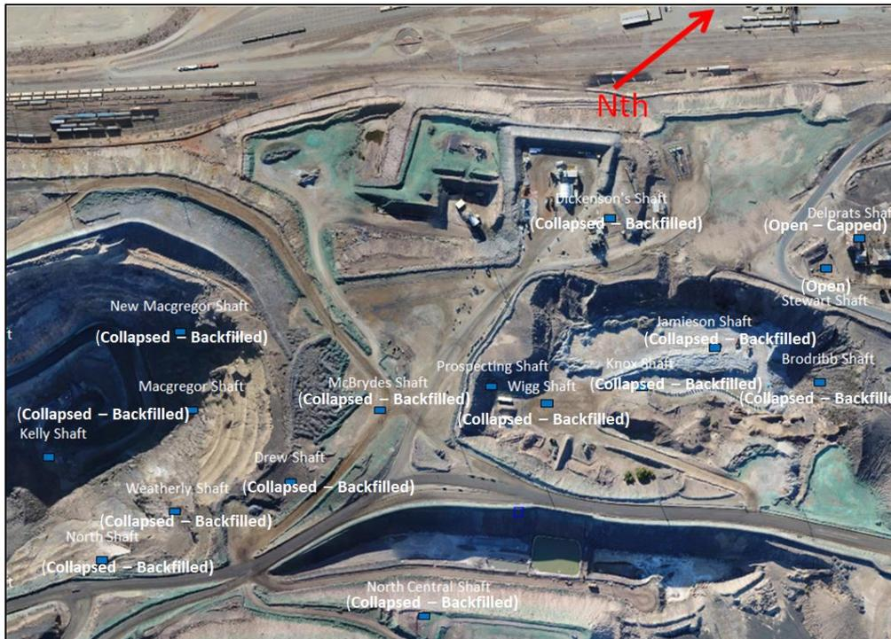
Figure 14- Surface shaft Collar locations and current status
