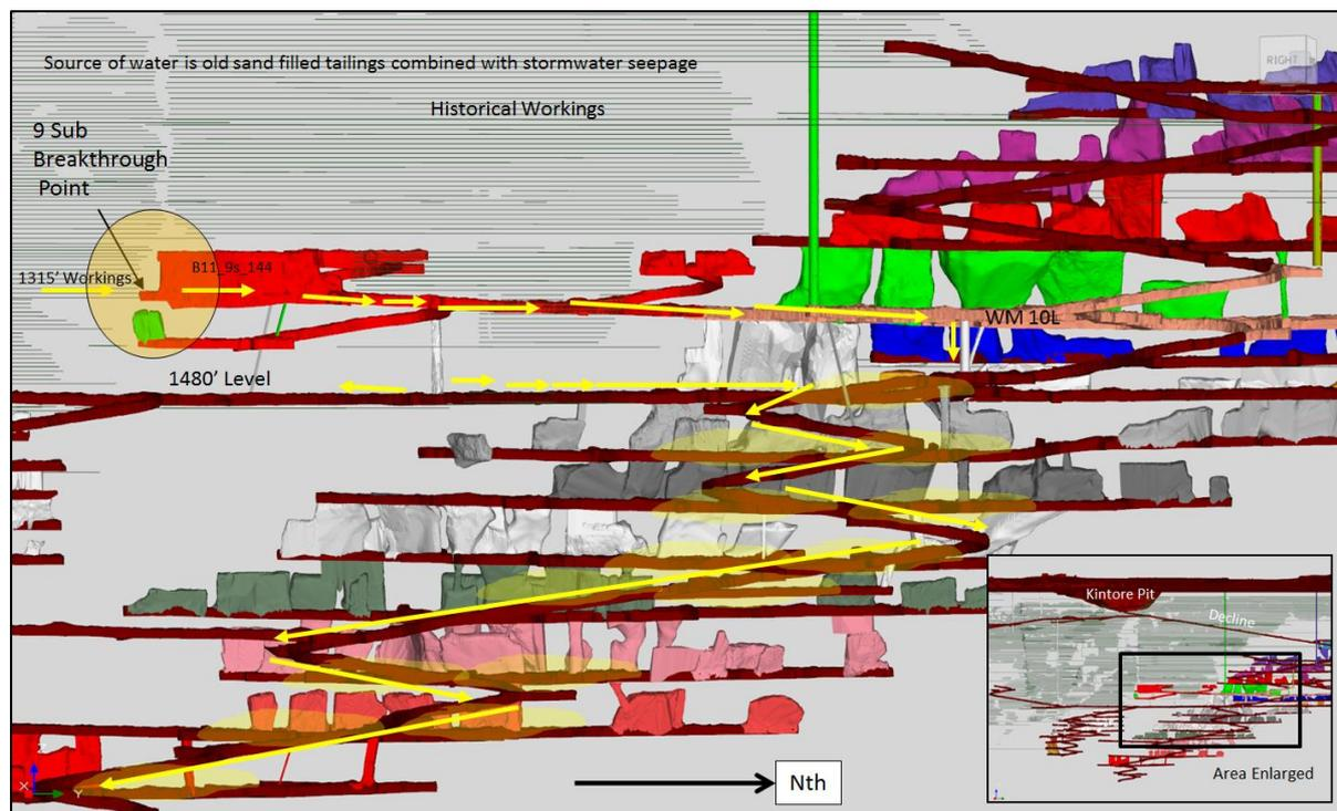
Figure 18- Potential WM fluid pathway from 9sub and connection with the 1315 ft workings
