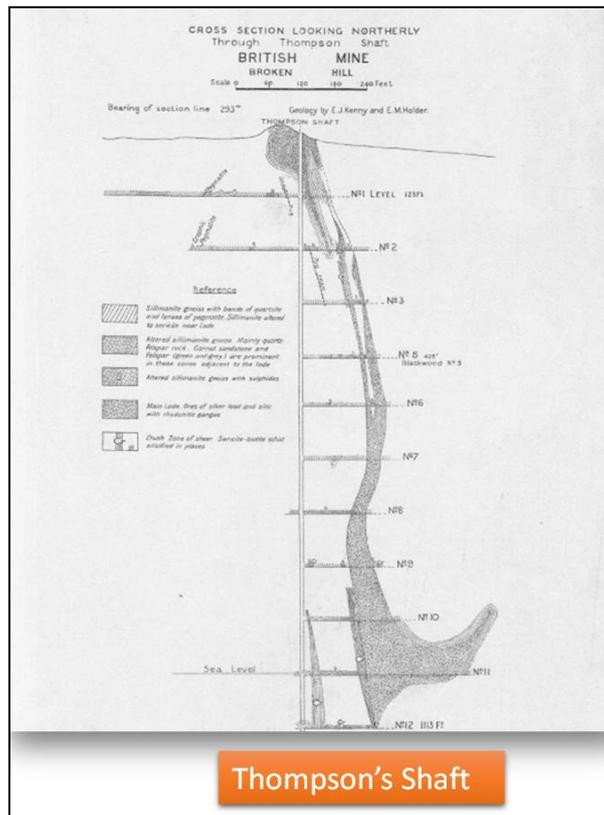
Figure 25- Thompson's Shaft (looking North) - 1922 (After Nixon, 2017)
