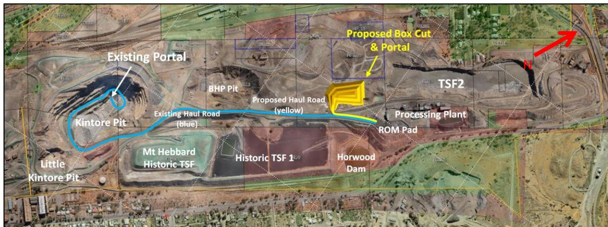
**Figure 1 – Site Plan showing proposed box cut location**
