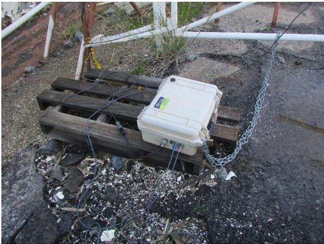
**Photo 25** – Blast monitor at monitoring point V6 (5 July 2023)
