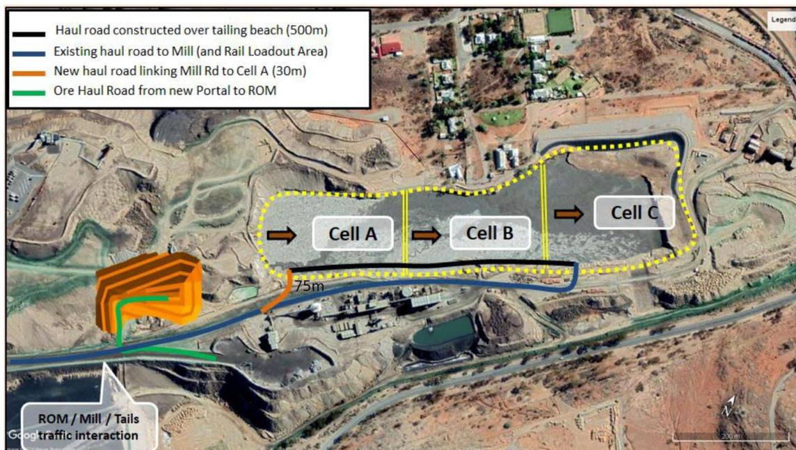
Figure 1.1: Indicative Layout Option for Tailing Harvesting (Source: BHOP)
