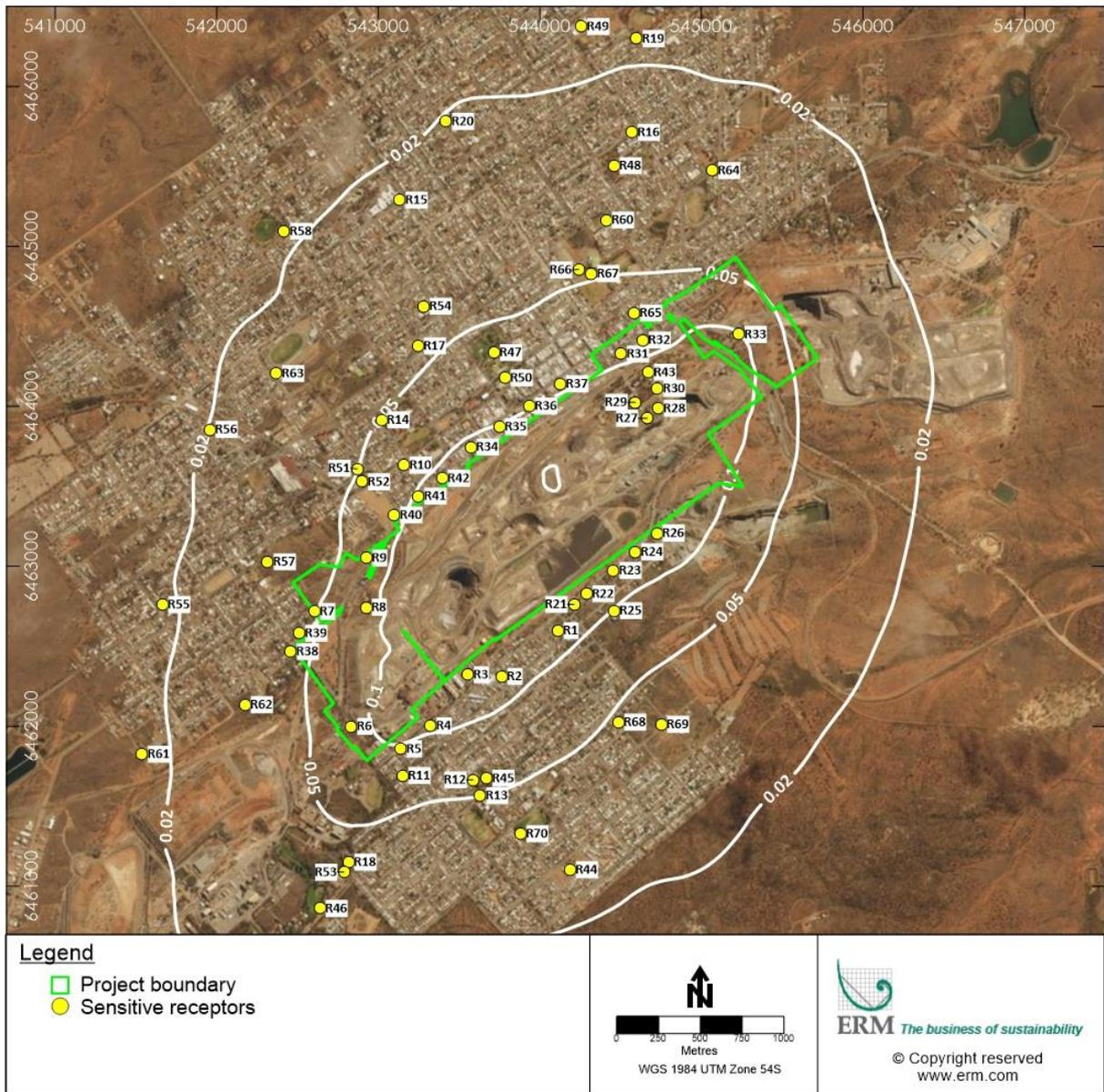
Figure I-15: Predicted incremental annual average PM<sub>2.5</sub> concentrations (µg/m<sup>3</sup>) for MOD6 operational scenario
