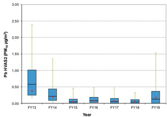
Figure H-6: Pb concentrations measured by HVAS2
