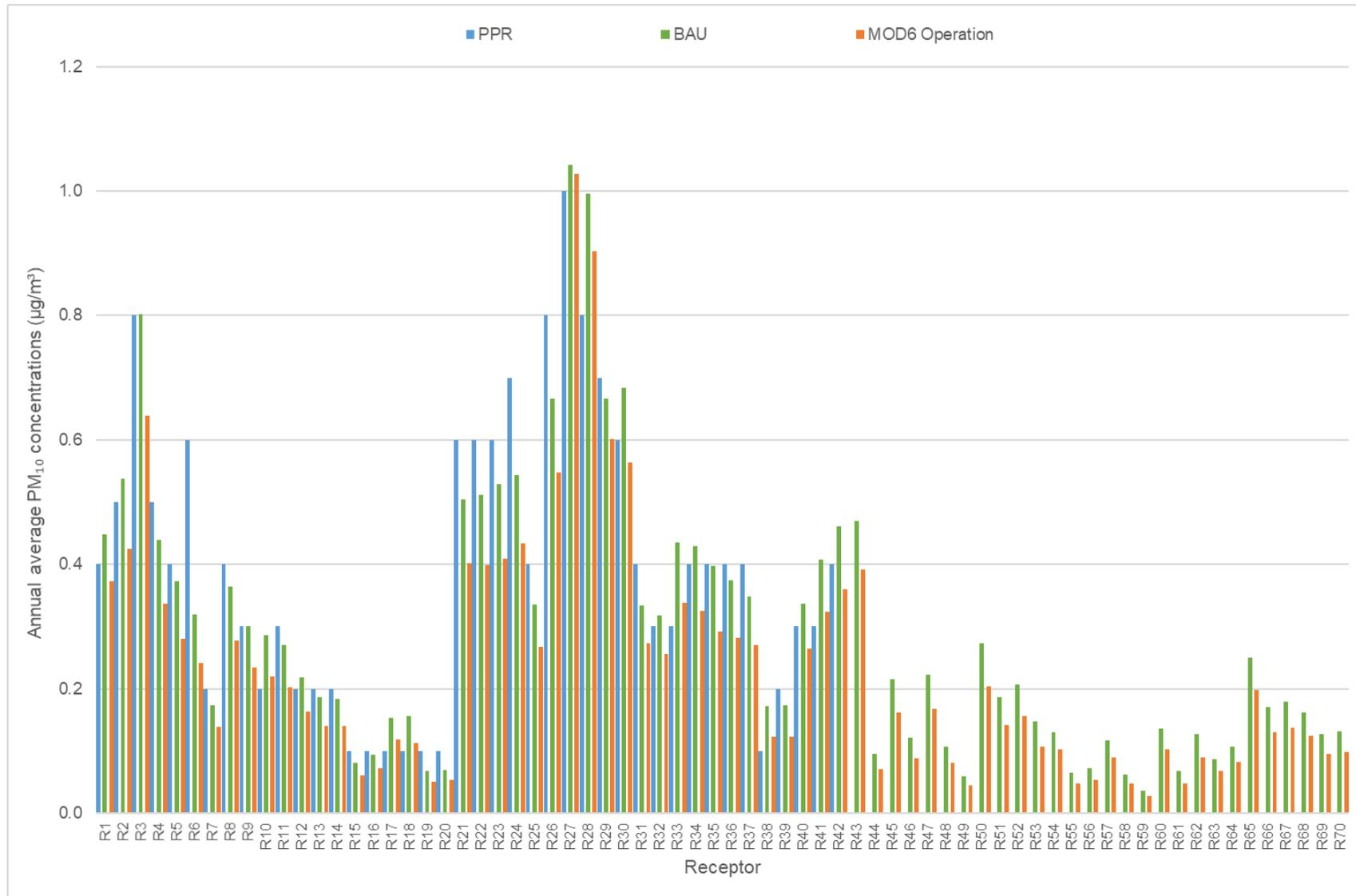
Figure E-4: Annual average PM<sub>10</sub> concentration for the MOD6 operational scenario, PPR assessment and BAU scenario
