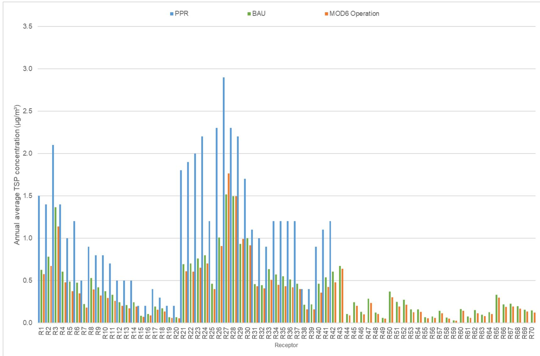
Figure E-3: Annual average TSP concentration for the MOD6 operational scenario, PPR assessment and BAU scenario
