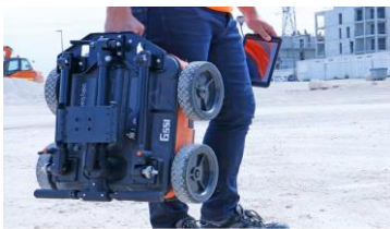
Ground Penetrating Radar
