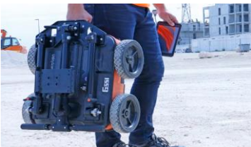
Ground Penetrating Radar
