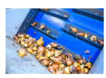
Rubber skirting-SBR high abrasion up to 6" wide and 1" thick
