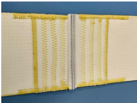
Representative sample of HSPY2 showing Double Plastic Spiral Lacing and 4 rows Kevlar stitching
