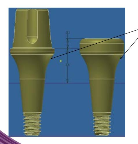
Notice how the healing abutment has the same emergence profile as the abutment.
