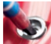
3. Pivot the tip back to easily pop out and remove the mounting insert from the housing.
