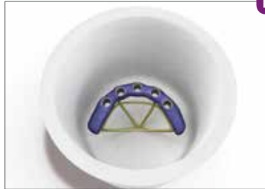
Castable ring with waxed framework.
