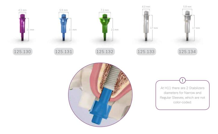
Insert the Guide Stabilizer after implant placement using the Neo Manual Screwdriver, fully engaging it until the physical stop. Hand torque it gently. Do not use the Guide Stabilizer when implant primary stability is lower than 20 Ncm.
