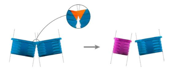
The GM NGS System allows flexible height sleeve position in the surgical guide. The two sleeve positions are 5 mm (H9) or 7 mm (H11), considering 9 and 11 mm from the upper part of the sleeve to the implant platform. For implant length of 18 mm a partial NGS technique is indicated.
