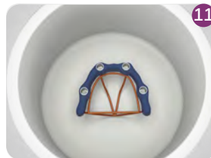
11 Castable ring with waxed framework.
